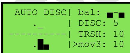
Lower the coil above the ground (6..10cm for small coil and 30..40cm for large coil) and press again **FAST ZERO**. If the ground signal is **mov3=5..6**, which little by little fades to 0..1, the coil moves left and right and the signals received are **mov3=8..10** due to the movement and the small changes in the ground signal. The sound threshold **TRSH=10**
